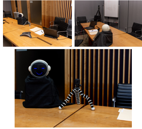
Fig. 7. The experimental setup, showing the head of Lil'Flo, across the table from the subject, a camera facing the subject from the direction of the head, a camera facing the subject and the head from the side, and the interviewer next to the head, with a control computer.
