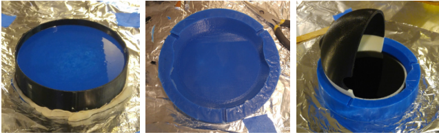
Fig. 5. On the left, making a mold to make the face screen. In the middle, the completed mold for the face screen, which is used to mold the translucent front screen. On the right, the translucent front screen being molded into a 3D printed model of the head. The material being used is a clear urethane with black colorant added.
