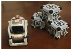
Figure 1: Anki Cozmo with its sensorized cubes
