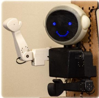
Figure 1: A picture of Lil'Flo with the arms attached. The arms still require paint but are mechanically complete.
